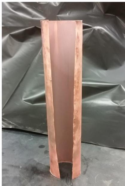
**Figure 12. Copper sheet electrowon from a surrogate cupric sulfate solution. The sheet was deposited on a stainless steel cathode, which was positioned along the inner periphery of the cylinder in Figure 11.**
