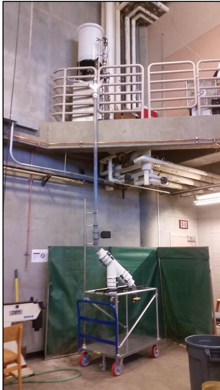
Figure 5. The Fourth Generation Continuous Flow Reactor System. Solution flows down through the vertical column from the head tank to the PVC wye. The electromagnet is seated near the top of the PVC wye.
