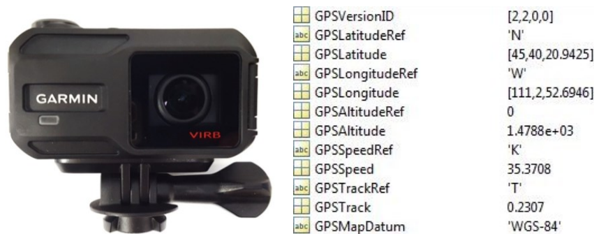
Figure 5. Garmin VIRB XE GPS-capable camera (left) and its GPS measurement recorded with the camera mounted on the dashboard of a car while driving at 35 km/h (right).
