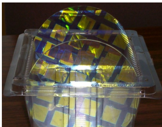
Figure 11. Four-inch wafers with microcavity craters and mirror coatings at 580 nm designed to measure common fluorescent protein markers. The wafers were designed and purchased on the AF STTR. The cross-hatch pattern allows access to a base ITO layer which provided electrical tuning of the liquid crystal layer. This next quarter they will be constructed into tunable LCAM cells and used to measure two fluorescent protein markers.
