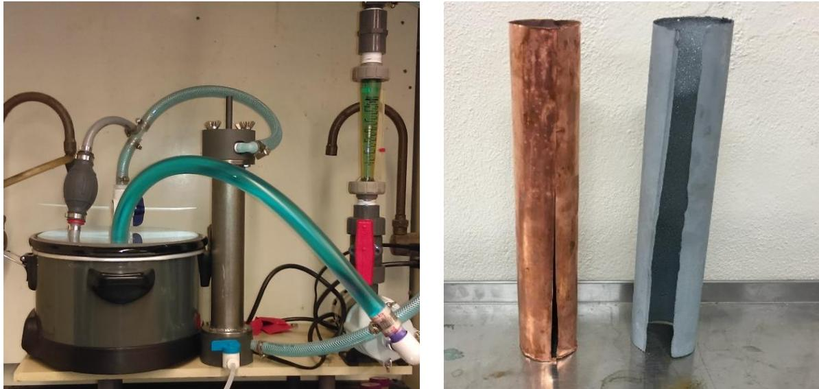
**Figure 10 – the laboratory electrowinning circuit. Electrowinning is a means of recovering metals from solution by reducing the ions and plating high-purity metal on a cathode. In this circuit, the actual electrowinning occurs in the cylindrical column at center. At right, copper and zinc sheets electroplated from surrogate sulfate solutions**
