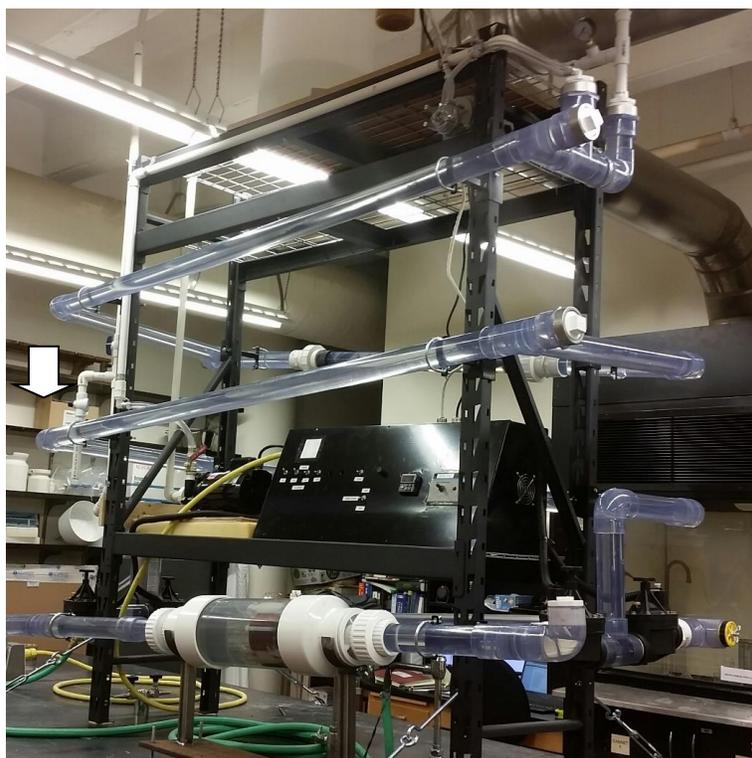
**Figure 7 – the 3<sup>rd</sup> generation continuous flow reactor. The white arrow in the photograph points to the in-line electromagnet module that captures and retains the magnetic nanoparticles without impeding the wastewater flow. This reactor has a 100 liter volume and solution flow rates range from 2 to 8 liters per minute.**
