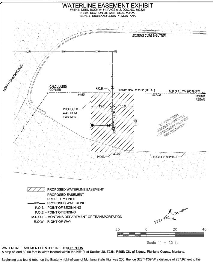
Beginning at a found rebar on the Easterly right-of-way of Montana State Highway 200; thence S23°41'39"W a distance of 237.92 feet to the centerline of the proposed Waterline Easement, the Point of Beginning; thence S66°43'57"E a distance of 41.00 feet to the Point of Ending.
