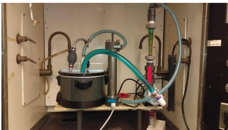
**Figure 11. Laboratory electrowinning circuit. Electrowinning is a means of recovering metals from solution by reducing the ions and plating high-purity metal on a cathode. In this circuit, the actual electrowinning occurs in the cylindrical column at center.**
